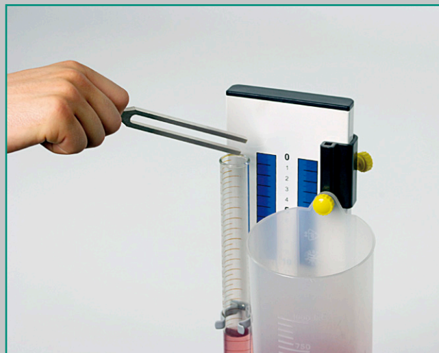
The resonance tube matching the wavelength of the incoming sound wave
