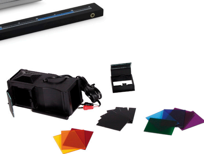
Ray box with coloured filters, slits, two side parts with mirror and transformer
