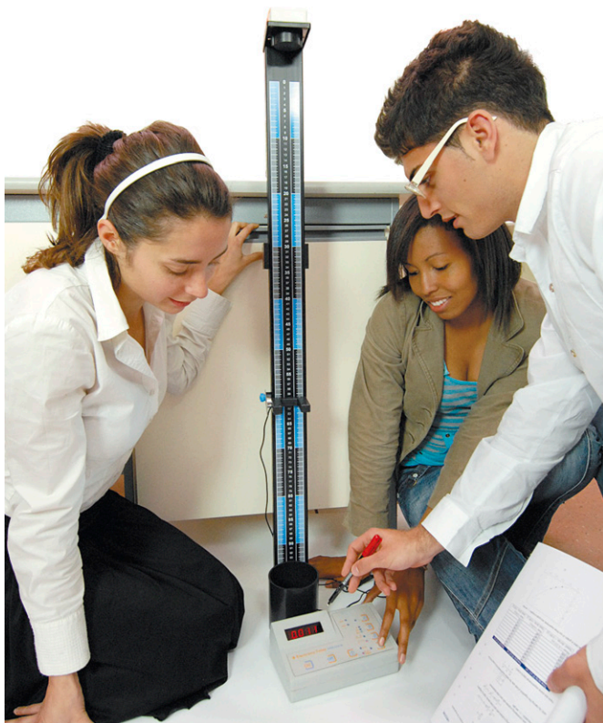
▲ Students acquiring data from Multiuse System in free fall configuration
