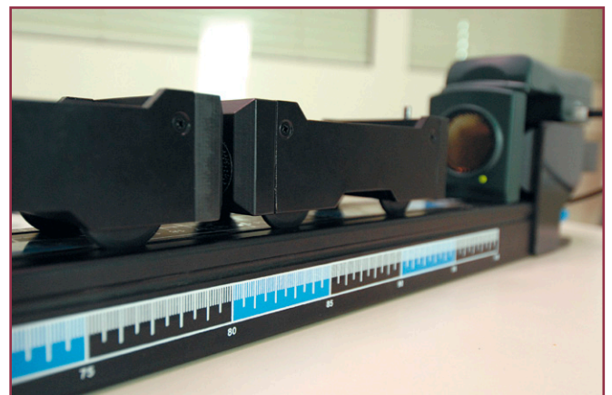
▲ Investigating collisions using a datalogger
