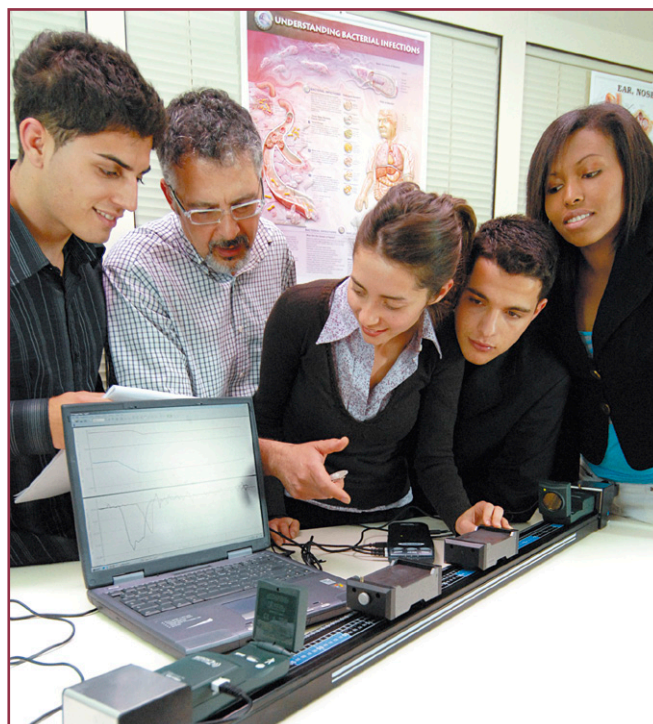
▲ Datalogger with motion detector used to acquire collision data with the Altay Mechanics Upgrade 1
