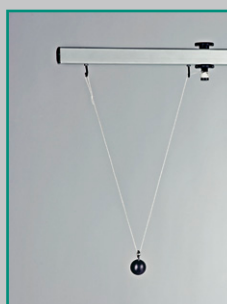
▲ Pendulum detail with bifilar suspension
