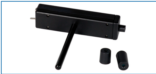
Solid state laser with cylindrical lens and polariser
