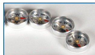
▲ Magnetic field lines of force demonstrated by series of plotting compasses
